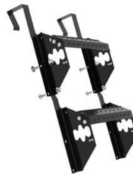
**Step 3:** Brackets can be attached together with M8x20 bolts, nuts and washers that are equipped with the system. Note that brackets are connected with round head square neck bolts.
