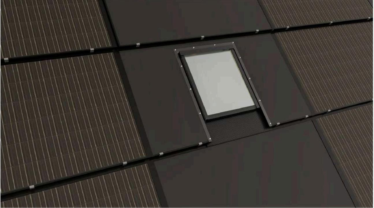
**Disclaimer:** The bottom roof window flashing must extend to another PV module. It should not lay between battens or be positioned on battens.
