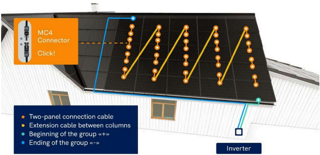
**Disclaimer:** It is mandatory to use only inverters with arc fault detection features.
