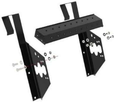
**Step 2:** Once the roof steps are fastened to the brackets, begin fastening the brackets together. The ladder can be extended to the necessary length.
